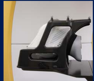
Fig. 4: A radiosurgery head phantom positioned with the frameless system. Ready for ExacTrac usage.
