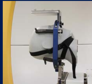
Fig. 3: A radiosurgery head phantom positioned with the invasive head frame. Ready for ExacTrac usage.
