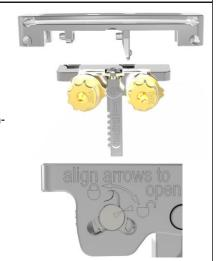
2. Insert the **A** and **B** pegs of the cutting slot into their corresponding holes of the adjustment unit.
