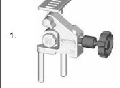
Screw **B4** out of **B3** and remove it from **B1**.
