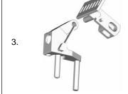
Turn B2 until leaf spring fits through slot of B1, and then remove B2 from B1.
