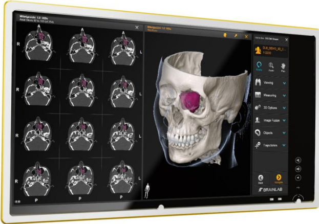
Illustration 1: Brainlab Buzz with interactive DICOM image viewer. The illustration shows a display from a computerised tomography scanner: a series of single layers on the left, and on the right the 3D visualisation of the data calculated "in real time" on the Buzz system. Objects can be highlighted for further planning of the procedure. In this example an object (a tumour in red) has already been defined and displayed in a 3D view.
